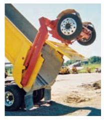
Large debris and bulky items exit quickly and completely with Crysteel's patented high-lift Hydraulic Tailgate which extends a normal tailgate to allow up to 6 feet of clearance when dumping!
