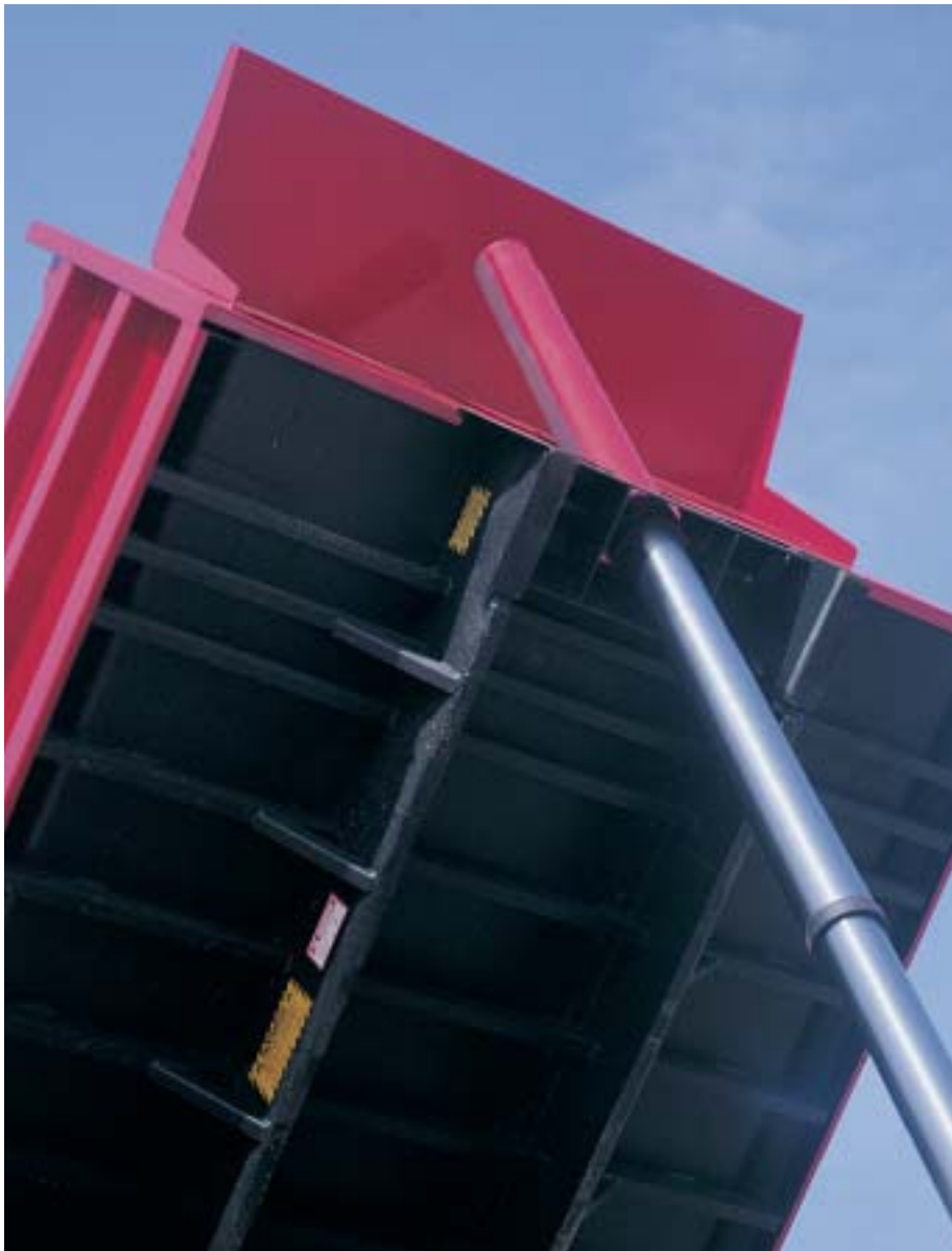
Crysteel Marathon's ingenious body mount lifts directly on the longbeams for efficient power delivery and superior stability, throughout the dump cycle.
