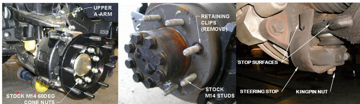
Figure 2 – Wheel Adapter Details
