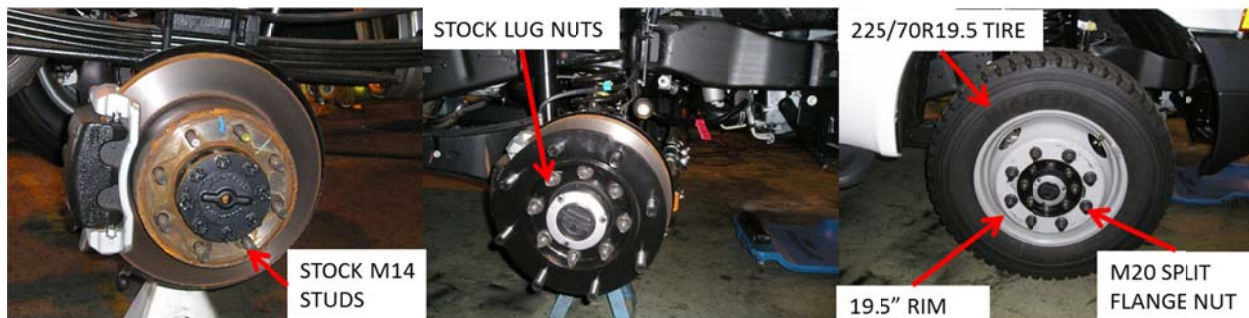
Figure 2 – Wheel Adapter Details
