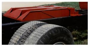
Hoist mounts low between the frame, meaning no notching crossmemebers under dump body.
